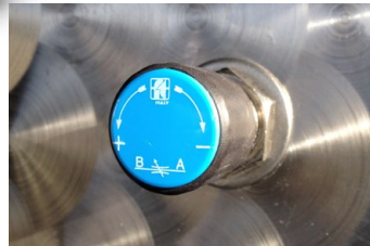
Range of water pressures (0-50bar/725psi) is available to operatives through the pressure control valve
