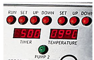
Timer can be programmed to run for up to one week
