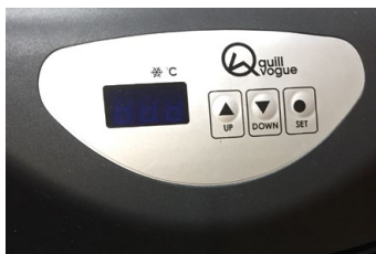
Cooler unit maintains water temperature below 30 degrees
