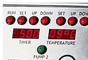
Timer can be programmed to run for up to one week and temperature can be set up to 99°C
