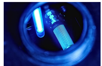
The Powder Wash is a "closed" system containing a 50 litre water tank with UV filtration system, making it environmentally friendly
