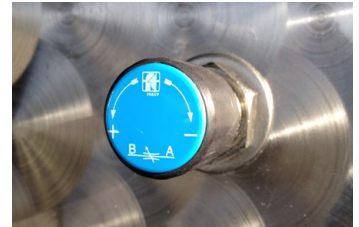
Range of water pressures (0-50bar/725psi) is available to operatives through the pressure control valve
